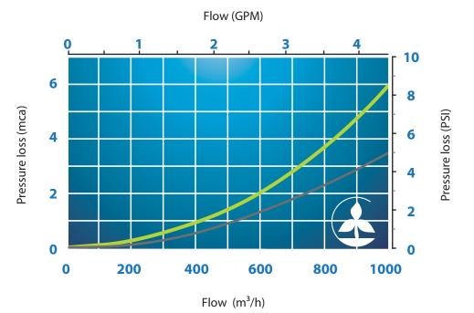
Pressure loss in a 47.2" (1.2 m) complete assembly with female and male fittings, flexible tube and ½" female adapter.
